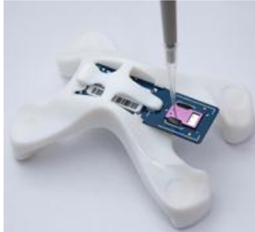
Veredus uses STMicroelectronics' lab-on-chip platform to detect avian flu.
