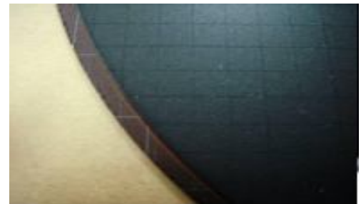
Molded wafer after die to wafer attachment
