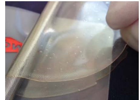
Flexible, transparent \sim 75\mu\text{m} thick freestanding toughened BCB film
