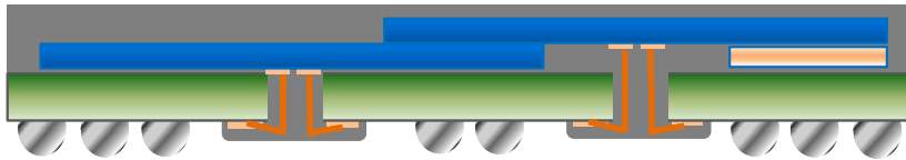
Dual Face Down (DFD) (side view)
