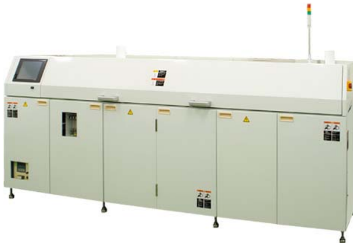
Conventional BGA reflow
