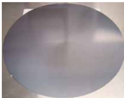
2 mil, 200 micron wafer with a 10 micron thickness coating of Ablestik WBC-8901UV.
