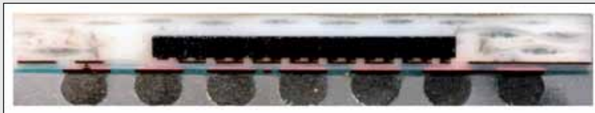
Figure 3. iBGA embedded die package WLP cross-section. (Courtesy of Imbera/Daeduck)
