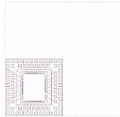
76L 6x6 mm TLA Terminal Pitch = 0.5 mm Total Signal Length = 93 mm Overall Thickness = 0.8 mm PCB Area Ratio = 0.25
