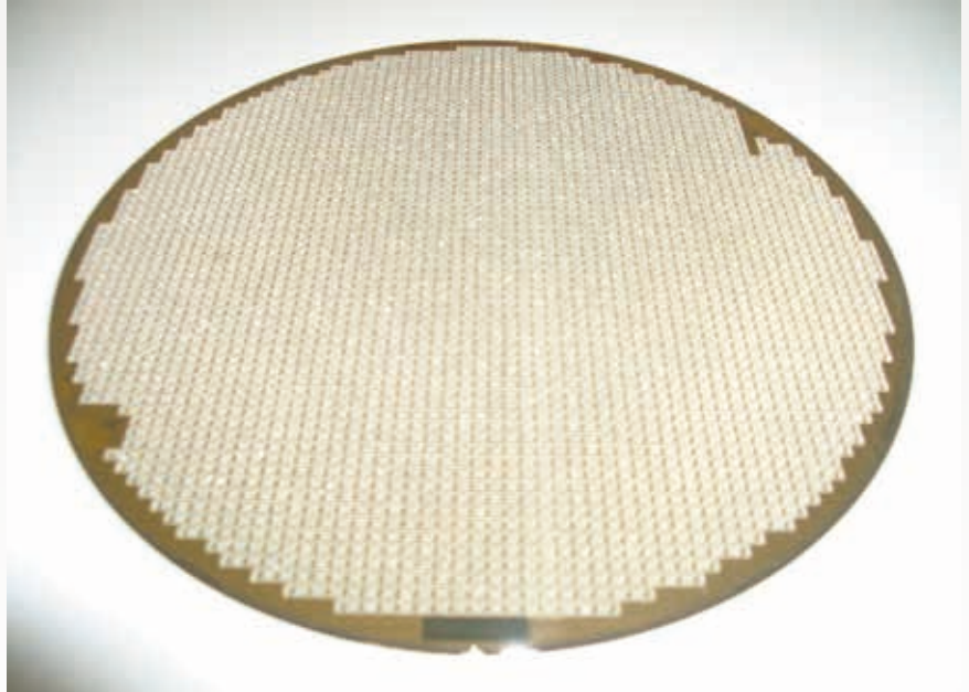
Wafer with electroless NiAu UBM.
