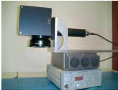
Figure 4. Early generation Q-Switch Pulsed Fiber Laser. Already more compact than the traditional Flash Lamp YAG in use well into this century. Note the elimination of the laser "Rail".
