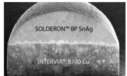
Figure 1. Cross-section of Cu pillars capped with SnAg capped pillar shows IMC compatibility.
