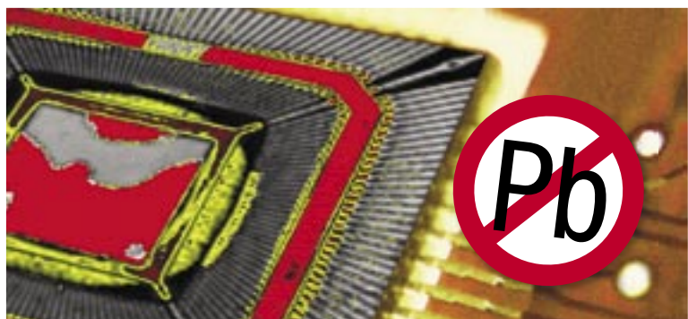
Acoustic Image showing delaminations (red)
