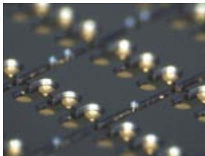
Figure 10: HyCap®U pad metallization on SMT side. Solder bumping is performed on wafer level by stencil printing.
