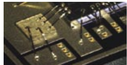
Figure 7: Active and passive device integration on HyCap®.
