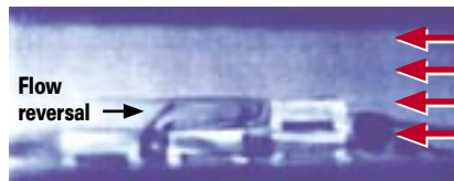
Figure 1: Water-based visualization of flow in an electronic board with the first component being twice the size of the others down-stream.
