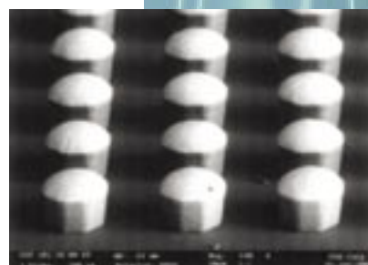
Array of copper bumps capped with solder.
