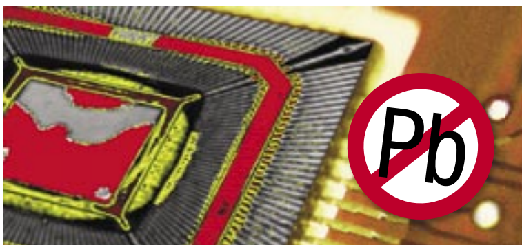
Acoustic Image showing delaminations (red)
