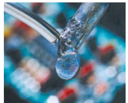
Tin-silver-copper-based solder alloys developed by Iver Anderson's research group are replacing lead-based solders for many electronic joining operations.
