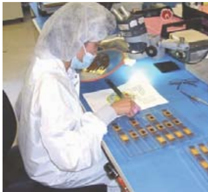
IC assembly using ceramic packages.
