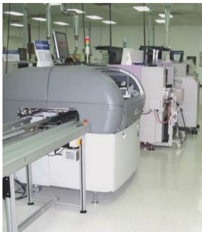
Fully automated lead free SMT optimized for SiP's and COB.
