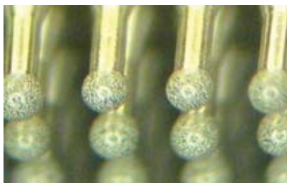
BD Paste Applied by Pin Transfer Process
