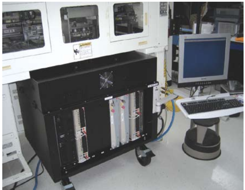
Figure 5. M-WeST docked to an NS-6040 Handler (Dual-Site configuration)
