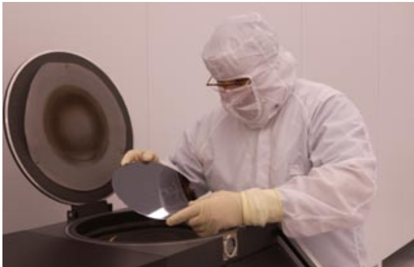
Figure 2. Research Engineer Bernd Scholz utilizing the reactive ion etcher in a process step of NanoBlock fabrication.
