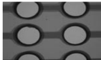
Figure 20. A view through 10 layers of a test coupon using XRF. No CAF filament could be found in the known failed areas.
