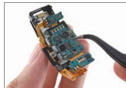
Figure 2. Samsung Gear Fit 2 teardown.
