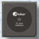
TEPBGA-2 Microcontroller (Engine Control Unit)
