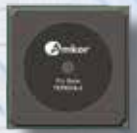
TEPBGA-2 Microcontroller (Engine Control Unit)
