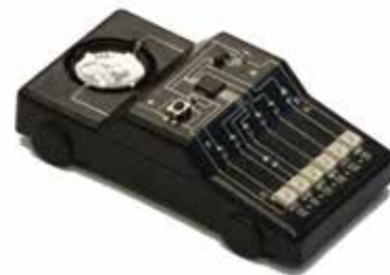
Figure 3. 3D MID Demonstrator Circuit - Ag on PA6 with added SMDs. (Source: Neotech AMT)
