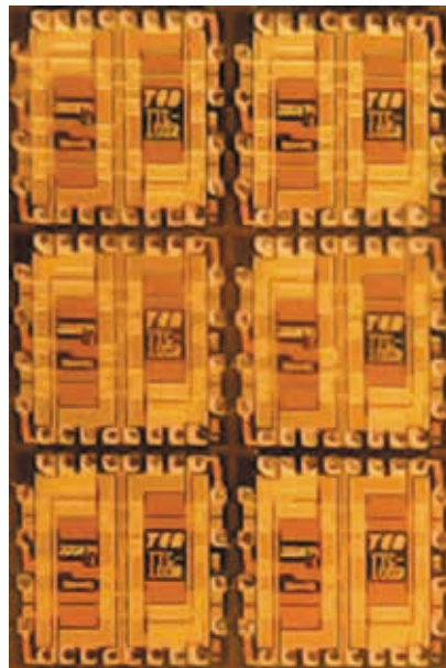
Figure 3B. TTC-1002 (2.5mm square Unit Cell) 2 x 3 Array.
