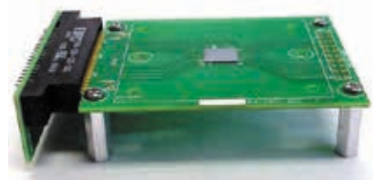
Figure 4A. TTV-4101 (TTC mounted on TTB) with mating edge connector.
