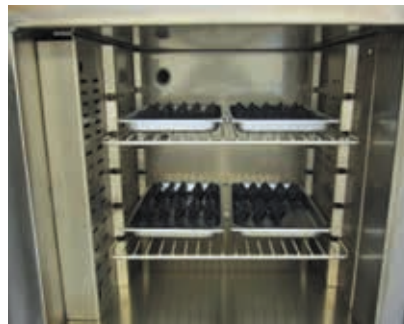
Environmental Life Test Chamber used to determine CTE mismatch issues.
