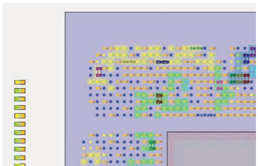
Figure 3: BGA ball array with signal, power, and ground planning completed and with some net assignments completed.
