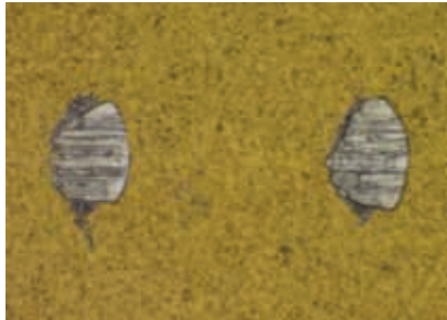
Figure 2. Sheared wire bonds.
