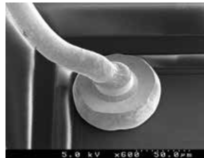
Fatigued/Deformed Wire Bond.
