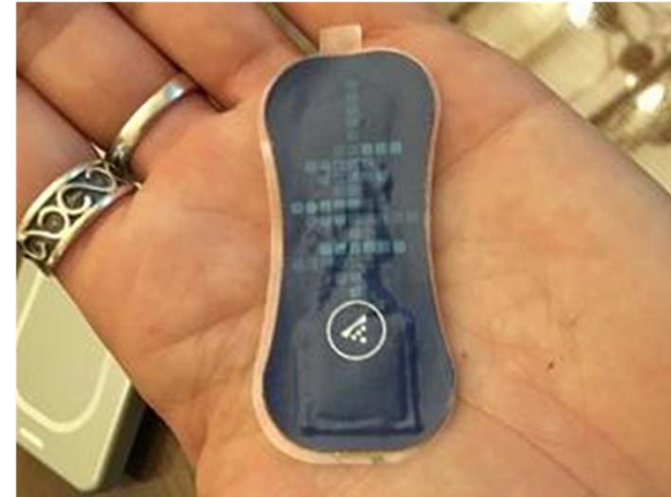
MC10's WiSP is a 300-micron-thin patch for monitoring electric-cardio activity.
