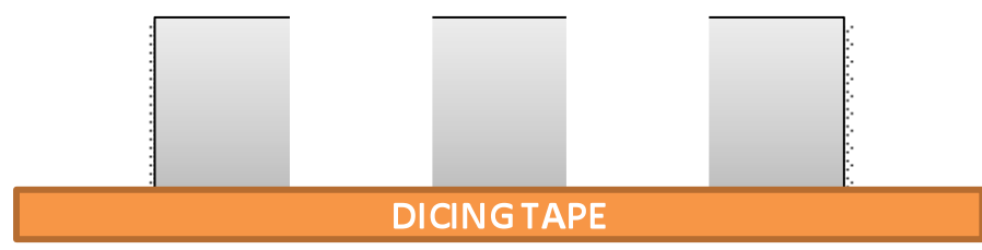
Mounted singulated die to dicing tape and frame and remove B/G tape
