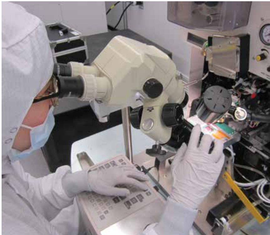
Wire bond process (shown left), coordinate measurement machine for incoming inspection (shown top right), and wire bond pull test (shown bottom right).
